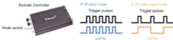
Receiver has two types, pulse and continuous, each for high frequency and continuous stimulation. The remote controller is compatible for both receivers, by switching the mode switch. Pulse receiver flashes at the same timing with trigger pulses, whereas continuous receiver alternates on and off upon a new pulse.
