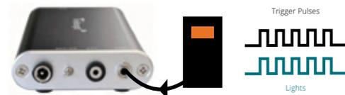
Remote controller accepts trigger signals from a stimulator, and sends the signals to the receiver. Synchronized light pulses are generated from the tip of the LED optic fiber (in pulse mode).
