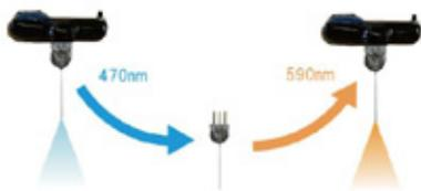
High brightness LED and optic fibers are coupled to achieve mW order light power at the tip. Colors can be changed just by swapping the LED optic fiber component.
