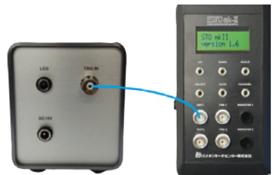
By the mode switch of LAD-1 LED Array Driver you can choose constant mode or trigger mode. In trigger mode, the Trg In BNC on the back panel is used for receiving trigger TTL pulses from a stimulator so that it enables time-controlled pulsed stimulation in-vitro.
