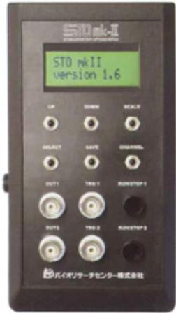
STO mk-II is a pulse generator developed for optogenetics. By connecting STO mk-II to TRG port on the Teleopto Remote Controller via a trigger cable, you can control the timing of light stimulation by TTL pulses. Pulses are defined by the parameters illustrated below.
